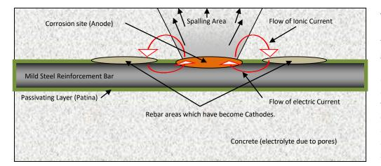
These corrosion cells increase in volume as the rust occupies a greater volume than the parent steel. This expansion creates huge explosive pressures on the surrounding concrete causing the concrete around the cell to crack and spall away from the surface
