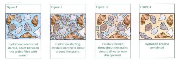
Steel reinforcement bars within concrete (pH value of 9+) benefit from the hydration process, as a passive layer is formed around the steel protecting it from corrosion. Providing the concrete is properly mixed and placed (well compacted and dense) this protection will last for many years.
