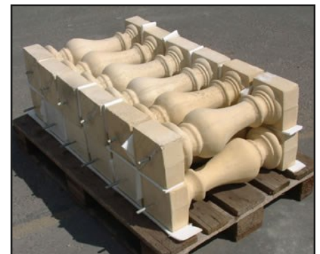
Concrete poured into pre formed moulds is used to form more ornate items such as these balustrades.
