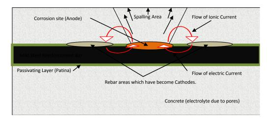
These corrosion cells increase in volume as the rust occupies a greater volume than the parent steel. This expansion creates huge explosive pressures on the surrounding concrete causing the concrete around the cell to crack and spall away from the surface.
